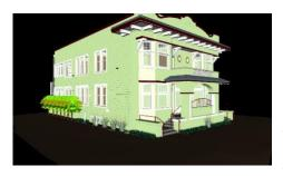
PAC\*SJ applauds FARO Technologies for its industry leading Laser Scanners, PointZ Taken for its on-site Laser Scanning Services and Digital Building Services Registration and Modeling Services that collaborated to create a 3-D point cloud and Revit Model of the Pallesen Apartment building. This effort provides a millimeter scale accuracy model of this one of kind building. This is the technology that ensures that a building can be
